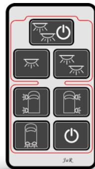
Control set is operable in a CAN bus system. That means it communicates only with using two wires (digital). Hence, the electrical installation is simpler and has less wires, compared to conventional installation (analog).
